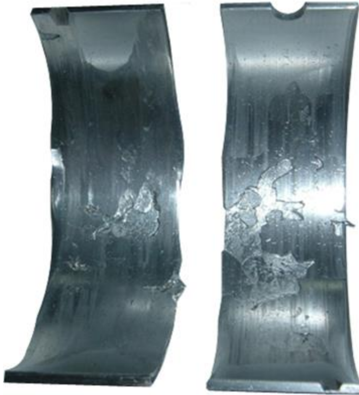
Fig.1 Fatigue of Aluminum Lining
