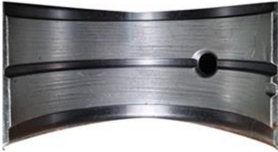
Fig.10 Damage Caused by Foreign Particles
