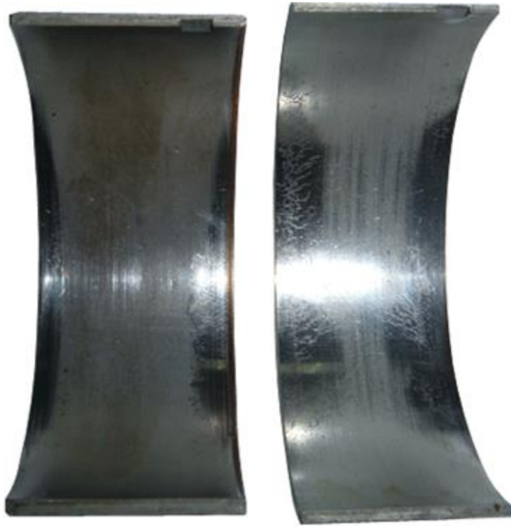
Fig.6 Local Wear due to Imperfect Journal Geometry
