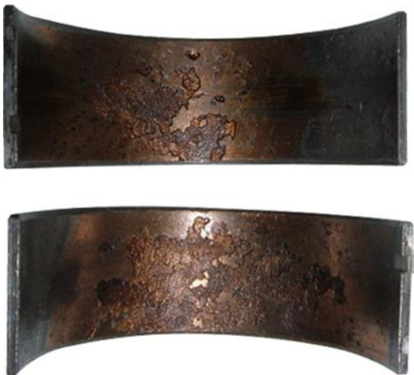
Fig.3 Fatigue of Bronze Intermediate Layer
