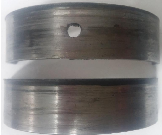
Fig.8 Spinning of Bearing in Housing
